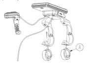
Now place the display on to the handlebar in the correct position, with two M4\*8 screws (C), tighten the display (B the clamps) into position. Torque requirement: 1N.m.
