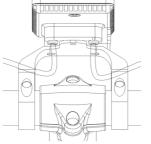
3. Open the clamp (D) on the controller pad and place it in the correct position (it is suitable for handlebar: ∮ 22.2).
