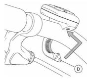
4. Using a M3\*10 screw (E) tighten the controller pad onto the handlebar. Torque requirement: 1N.m.
