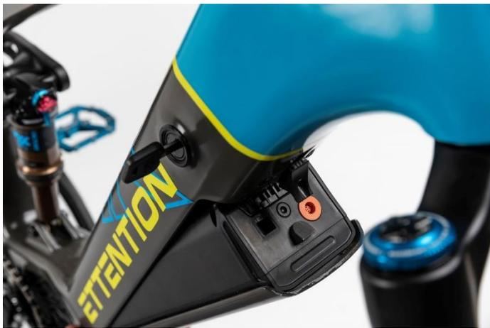
competing formats are considerably less space-efficient. A 36V battery’s 10S4P or 10S5P arrangement only manages 63% space utility, a 48V battery’s layout (13S3P, 13S4P or 13S5P) reaches no more than 65% – plus, that “high-end” 48V battery leads to a very wide package which conflicts in particular with the requirements of state-of-the-art downtube integrated batteries.
